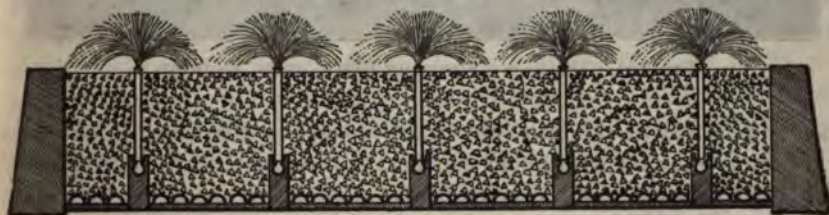
FIG. 128.—TYPICAL SECTION OF A SPRINKLING FILTER.
