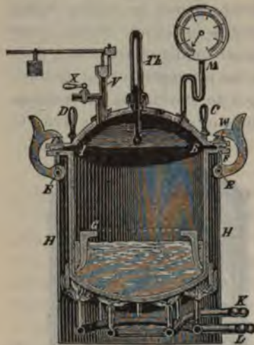
FIG. 156.—SECTION THROUGH AUTOCLAVE.
