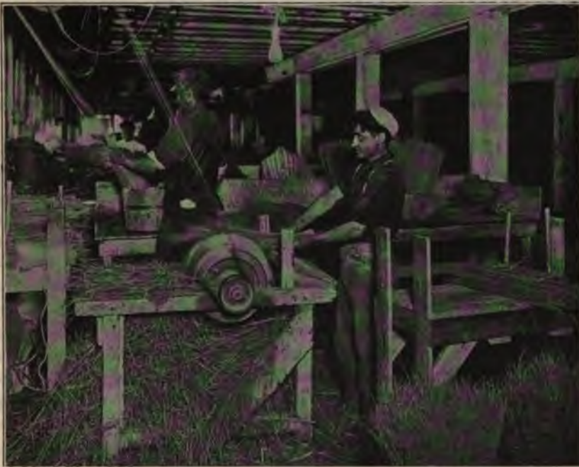
FIG. 150.—A VERY DUSTY TRADE—DRUM WITH NAILS WHICH COMBS OUT THE SMALL PIECES OF BROOM CORN. (Mass. State Board of Health.)
