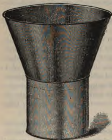
FIG. 164.—FLARING TOP TIN BUCKET FOR GENERATING FORMALDEHYD BY THE PERMANGANATE METHOD. Height 15 inches, diameter 10 inches at base, 15 inches at top of flare.
