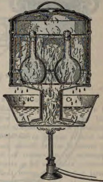
FIG. 155.—SECTION THROUGH ARNOLD STEAM STERILIZER.
