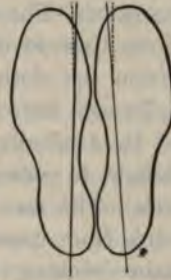
FIG. 179.—SHAPE OF U. S. MILITARY SHOE. A-B, Meyer's line. The dotted line shows slight deviation outward so as to fit the average foot accustomed to shoes.
