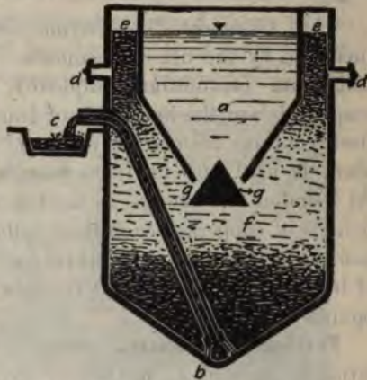
FIG. 122.—TYPICAL SECTION OF AN IMHOFF TANK.
